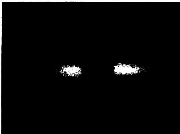
FIG. 2. Anisotropic scattering in the x - z plane. The concentration of the sample is \phi = 5\% and the dimensionless sample thickness is L/D = 25 . The optical anisotropy is a result of particle chaining along the z direction (vertical direction). The field (4 G) is applied adiabatically.
