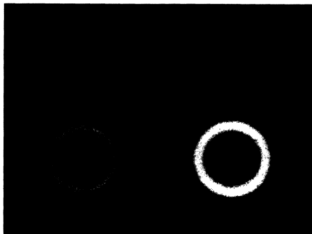
FIG. 4. The scattering intensity distribution in the x - y plane. The concentration of the sample is \phi = 5\% and the sample thickness is L/D = 25 . The magnetic field is applied adiabatically.
